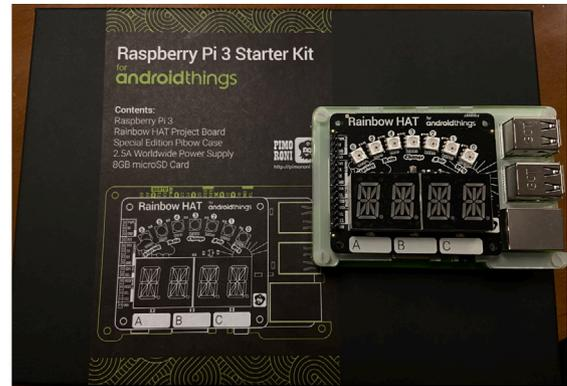
Fig. 9. Raspberry Pi 3 Starter Kit for Android Things.
