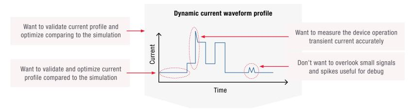
Figure 1. Example of low-power device and measurement requirements
